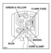
If you fit your own plug, the colours of the wires in the mains lead of your appliance, may not correspond with the markings identifying the terminals in your plug, proceed as follows:
